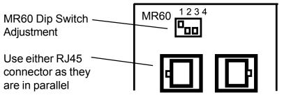
The rear of the MR60 is shown. Because one to three MR60's can be connected or daisy chained to the same cat 5 wire, the keypad position on the wire must be selected using the dip switch. The two MR60 RJ45 connectors are in parallel. Only one dip switch slider should be on and the other two off (#1 is shown on in this example). The MR60 1-2-3 dip switch positions correspond to MVP44a keypad ports and speaker outputs A3 or B1-B2-B3.
